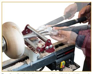
The rollers allow the tool to move smoothly, whilst being held securely
