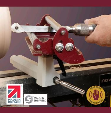
The Robert Sorby SteadyPRO is a very easy to use jig that gives additional tool support when bowl turning, hollowing and when doing spindle work.
